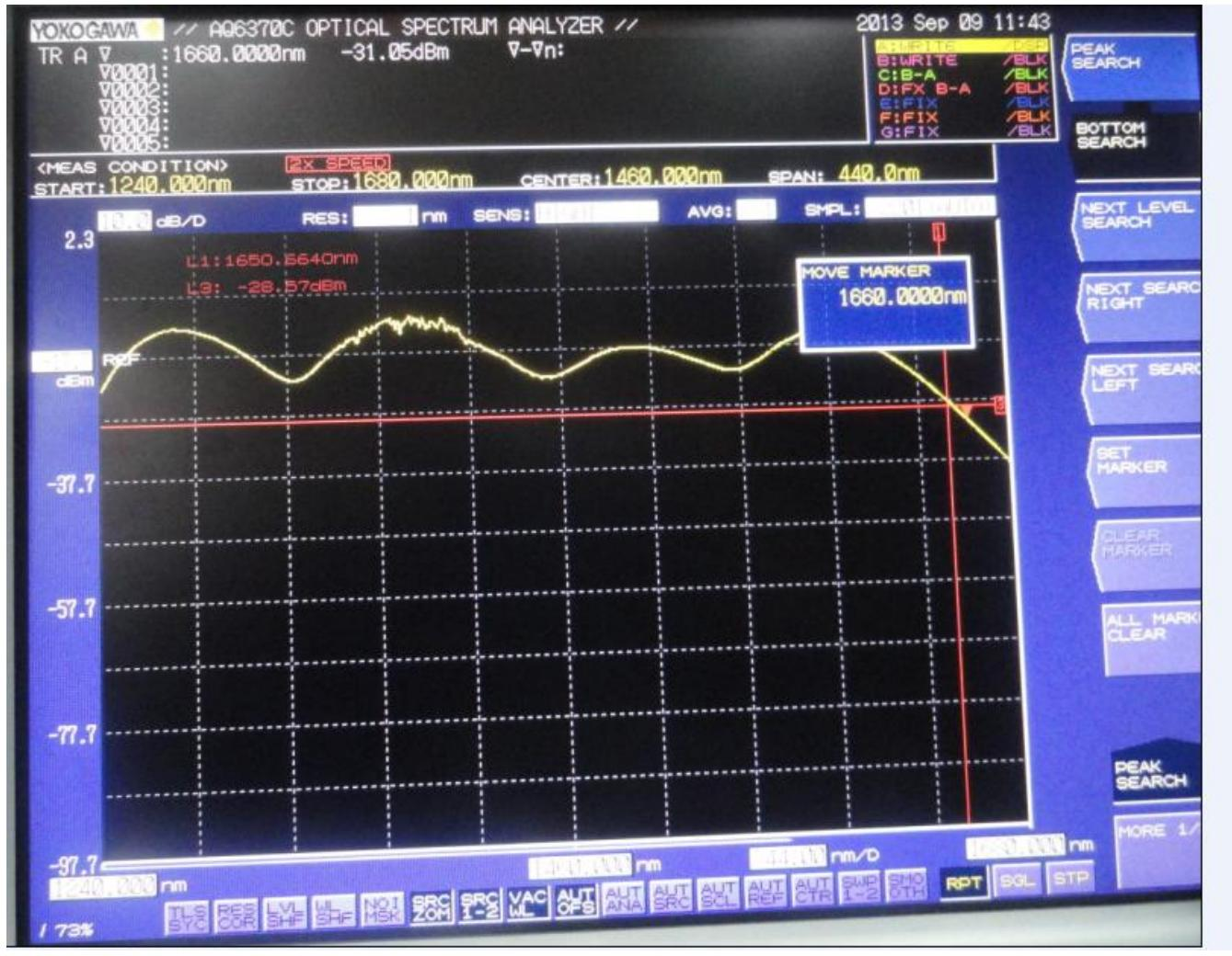
**-25dBm/nm spectrum;**      **1350nm~1420nm is at HO absorptioin , The rippler is  $\leq +0.2\text{dB}$**
